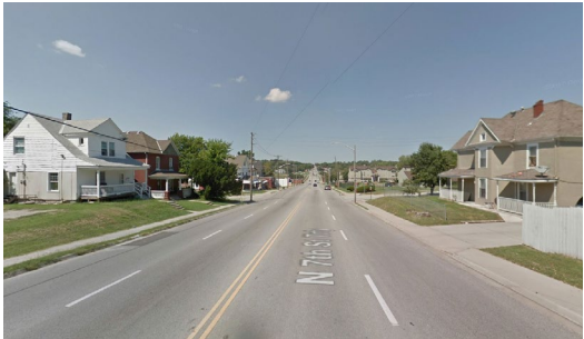
7th Street Existing Lanes: 4-5 Capacity (ADT): 38,000 Excess Capacity: 31,980 Future Lanes: 3 Capacity (ADT): 21,900 Excess Capacity: 15,880
