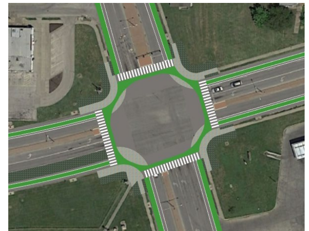
Above, an existing aerial of 18th and Parallel and below, a proposed graphic showing the installation of bicycle and pedestrian facilities
