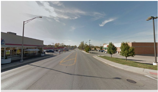
State Avenue Existing Lanes: 4 Capacity (ADT): 30,400 Excess Capacity: 22,185 Future Lanes: 3 Capacity (ADT): 21,900 Excess Capacity: 13,685
