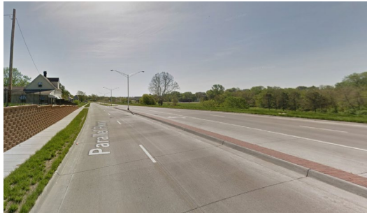
Parallel Parkway Existing Lanes: 5 Capacity (ADT): 40,500 Excess Capacity: 28,655 Future Lanes: 3 Capacity (ADT): 23,300 Excess Capacity: 11,455
