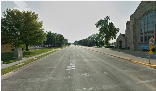
Washington Boulevard Existing Lanes: 5 Capacity (ADT): 40,500 Excess Capacity: 30,845 Future Lanes: 3 Capacity (ADT): 23,300 Excess Capacity: 13,645
