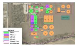
• Kaw Point Biosolids Project – Rehabilitate current structures and install new equipment to restore the digestion process allow for the handling of sludge which is currently landfilled, which is not cost efficient and will likely not be an option in the near future.
